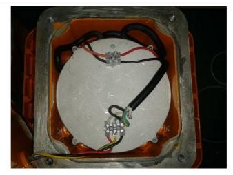
(This photo is close to the real product, pls reference it mainly when wiring. In the photo, the white and red wires are live lines, the black wires are neutral lines and the green/yellow is ground line) Connect each line rightly with the input terminal of the cable from the AC power source respectively by using screwdriver.
